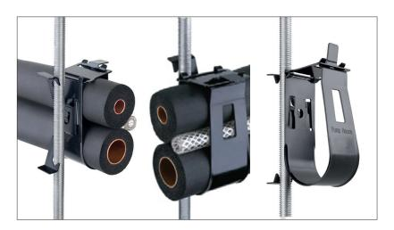
These clamps support a pair of flow and return insulated copper air conditioning pipes on either M8 or M10 threaded rod. By simply squeezing the tips together the spring steel rod hanger can be fitted or adjusted in seconds, even after the refrigerant pipes have been installed.
